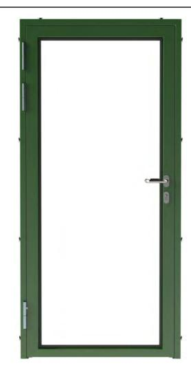
Once frame is secure hang door leaf and adjust hinges to allow ironmongery to operate correctly. Hinges can be adjusted vertically up to 5mm each by means of screw adjuster in top of hinge and horizontally by means of supplied hinge packer/shims.
