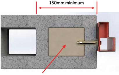
Void to be backfill d with suitable materials to a depth of at least 150mm.
