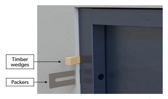
Drill through the top fixin port of the hinged jamb into the masonry/steelwork to accommodate the required fixing (the latter into steelwork will also require the steel work to be tapped prior to applying the fixing)
